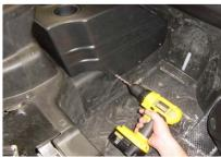
Once the enclosure is in place, press down on the top of the enclosure to insure it is snug against the center hump, while still applying pressure to the top of the boxdrill the 6 mounting holes using a 11/32 drill bit
