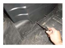
Then thread one Acorn nut and washer onto the threaded rod, insert from the passenger side and slide through the center hump so that the treaded end comes through the hole on the driver side, repeat this for the other mounting locations. Once all the threaded rods are inserted put a washer, then an Acorn nut on the remaining side, Using 2 - 14mm wrenches tighten the Acorn nuts. They need to be snug, **DO NOT OVER TIGHTEN**
